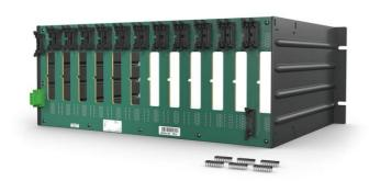
The EMC-DB02 Evolution Mounting Chassis, Divisible Bus, FRONT mounting rail provides mounting space for up to twelve (12) evolution modules within the same space as an MMU. The EMC chassis replaces MMU12 or MMU22 Module Mounting Units. The chassis has been designed so that I/O cables originally attached to the MMU can be attached in the exact same location once the EMC has replaced the MMU.
