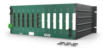
The EMC-SB02 Evolution Mounting Chassis, Single Bus, front mounting rail provides mounting space for up to twelve (12) evolution modules within the same space as an MMU. The EMC chassis replaces MMU12 or MMU22 Module Mounting Units. The chassis has been designed so that I/O cables originally attached to the MMU can be attached in the exact same location once the EMC has replaced the MMU.
