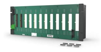
The EMC-SB01 Evolution Mounting Chassis, Single Bus, rear mounting rail provides mounting space for up to twelve (12) evolution modules within the same space as an MMU. The EMC chassis replaces MMU11 or MMU21 Module Mounting Units. The chassis has been designed so that I/O cables originally attached to the MMU can be attached in the exact same location once the EMC has replaced the MMU.
